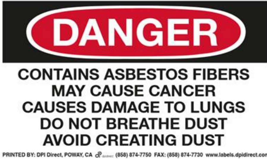
EXAMPLE Asbestos Label
