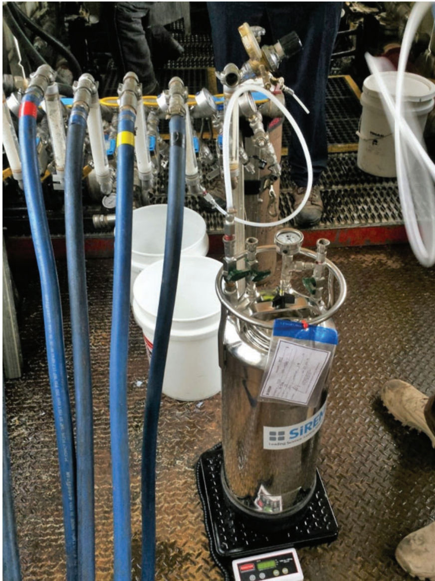
An EISB injection manifold attached to a KB-1® Plus vessel and scale. The blue injection lines on the manifold deliver EVO solution and KB-1® Plus to individual injection wells.
