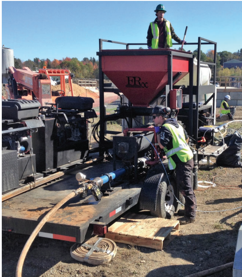
An injection contractor's amendment mixing and injection rig, equipped with a hopper for granular solid amendments, a guar mixing tank, an auger mixer, and a progressive cavity pump.
