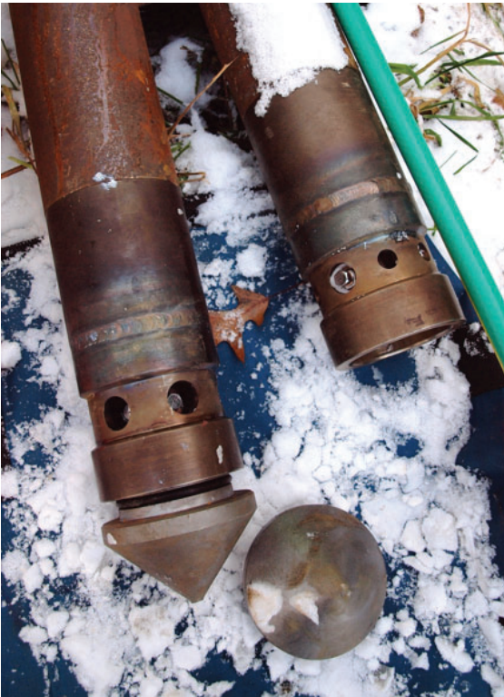
A dual-fluid injection tip for DPT jet injection attached to 3.5-inch Geoprobe rods.
