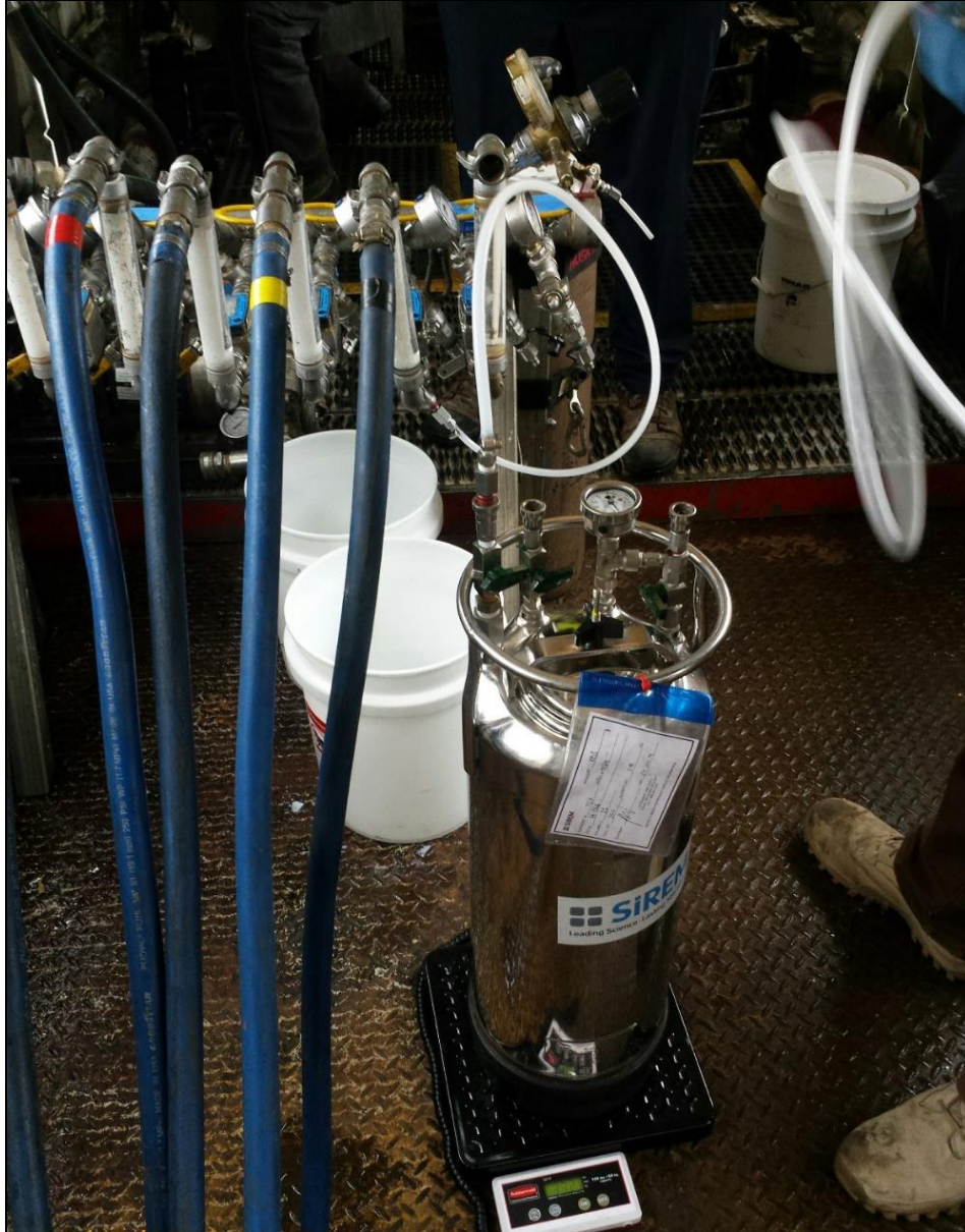
Figure 11. Photograph of an Injection Manifold Attached to a KB-1 ® Vessel and Scale
