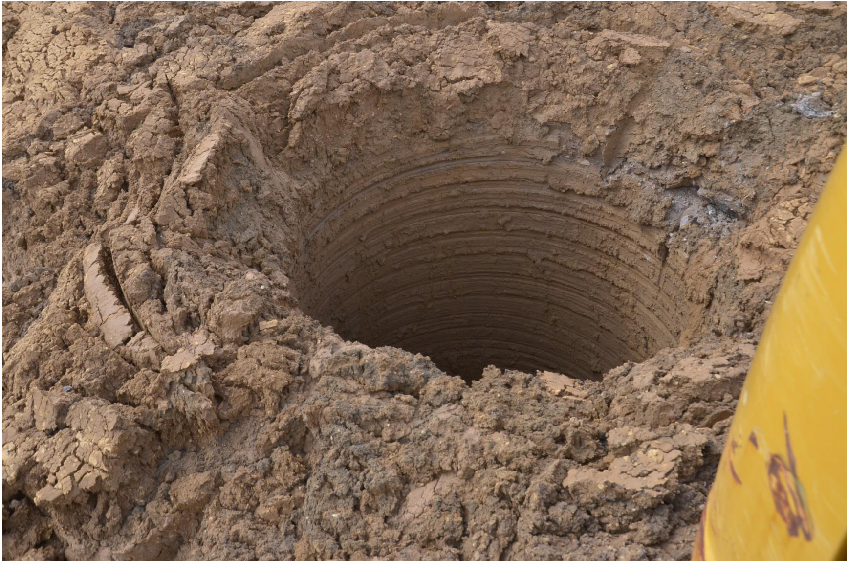
Figure 24. Photo Indicating Hole in the Ground Left by Soil Ejection Resulting from a Particularly Strong Soil Burp (Hole was ~ 8 ft wide—Taken on April 20, 2015)
