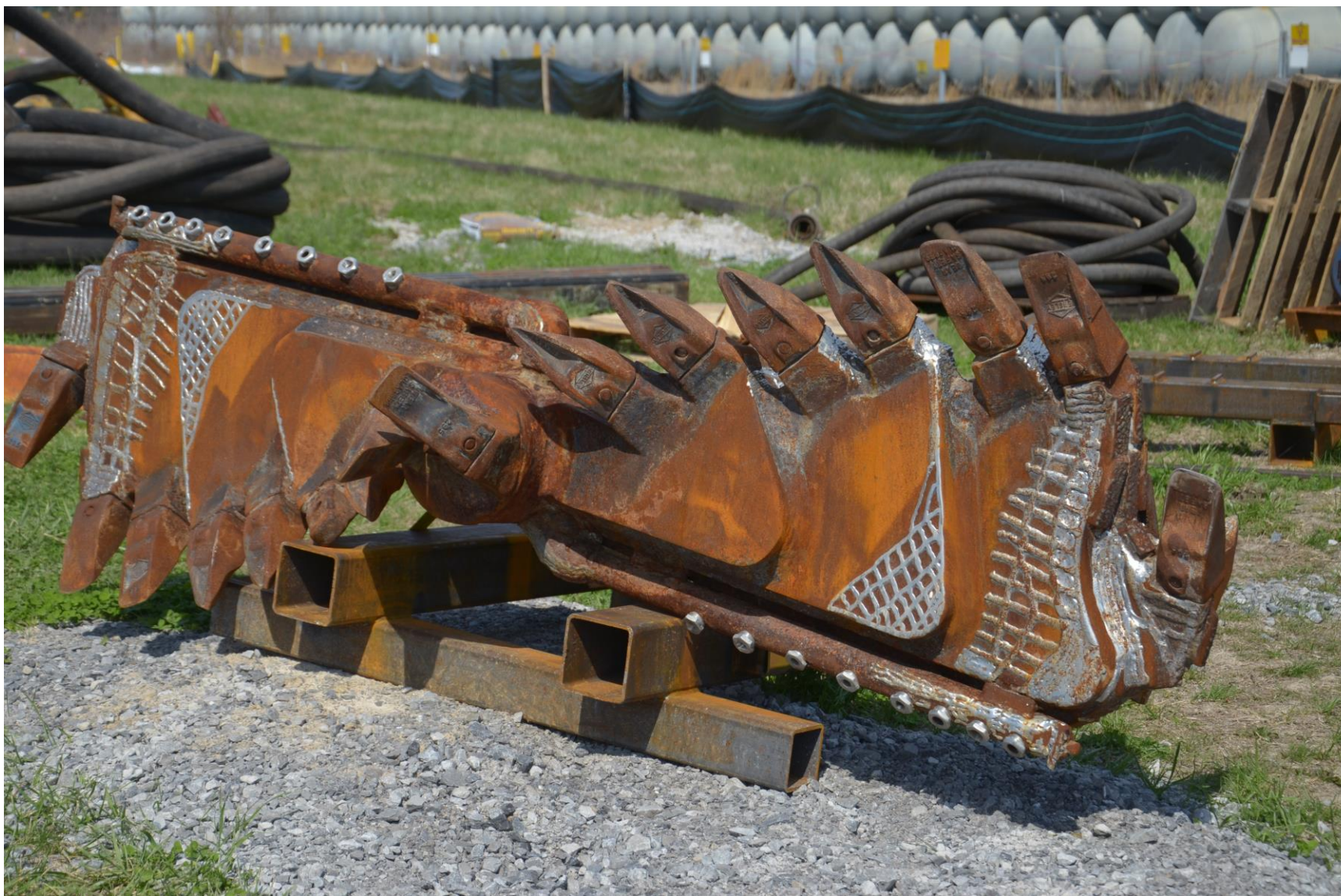
Figure 29. Multi-Blade Rotating Mixing/Injection Tool (Looking Northwest on March 31, 2015)
