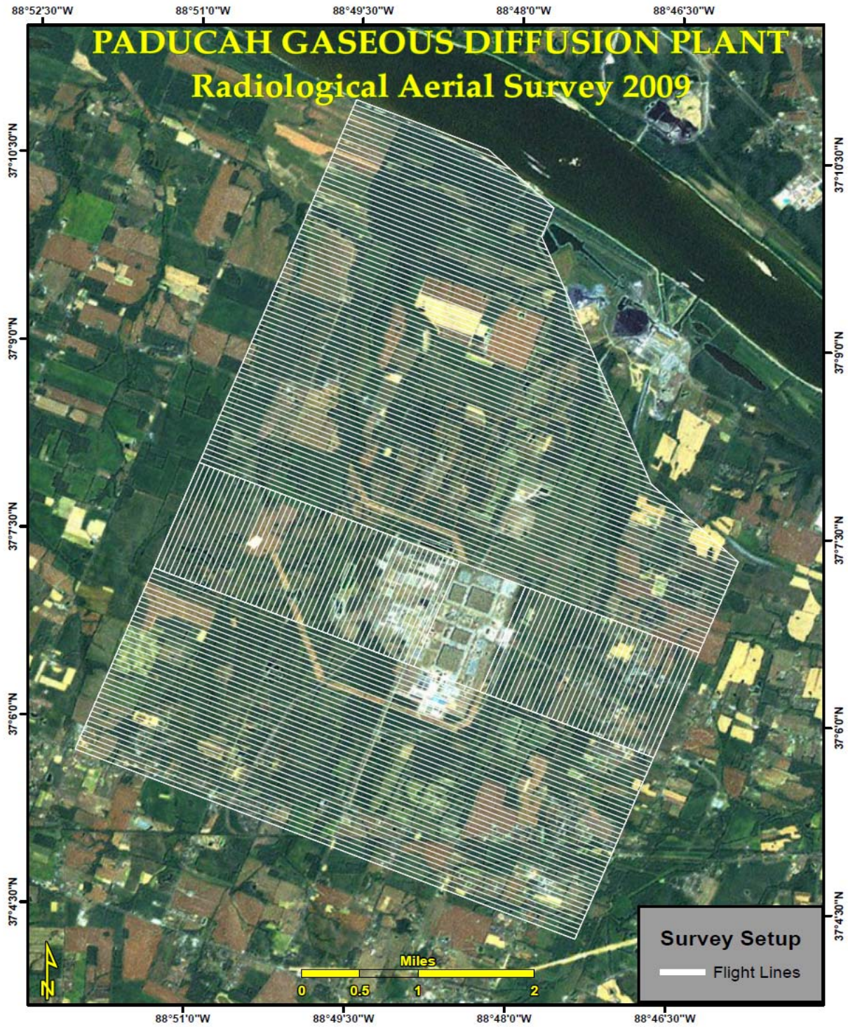
Figure 1: Survey Setup for PGDP Aerial Survey. (The open region in the center of the survey area was a restricted flight zone.)
