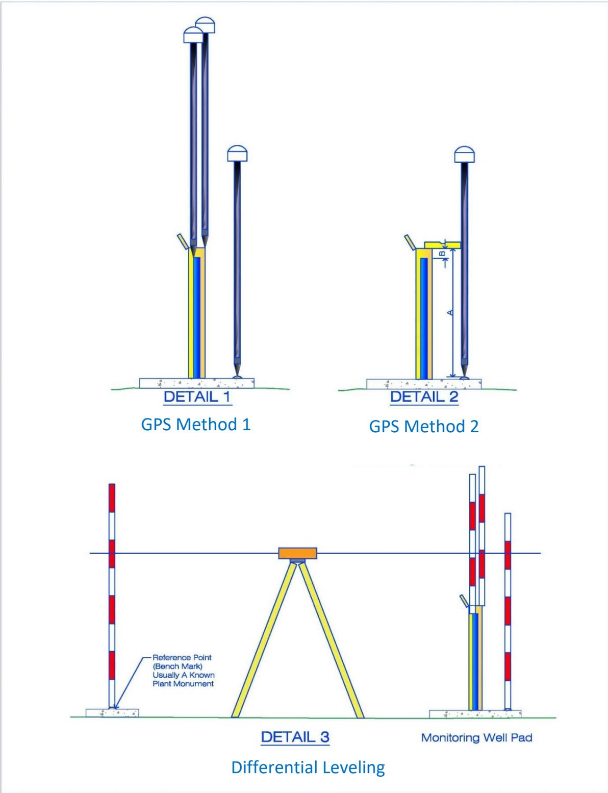
**Figure 1. Schematics of Surveying Methods**
