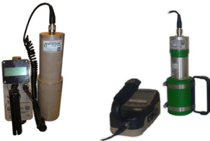
Figure 1: Sodium Iodide Detector Systems. [2x2 (left), 3x3 (right)]
