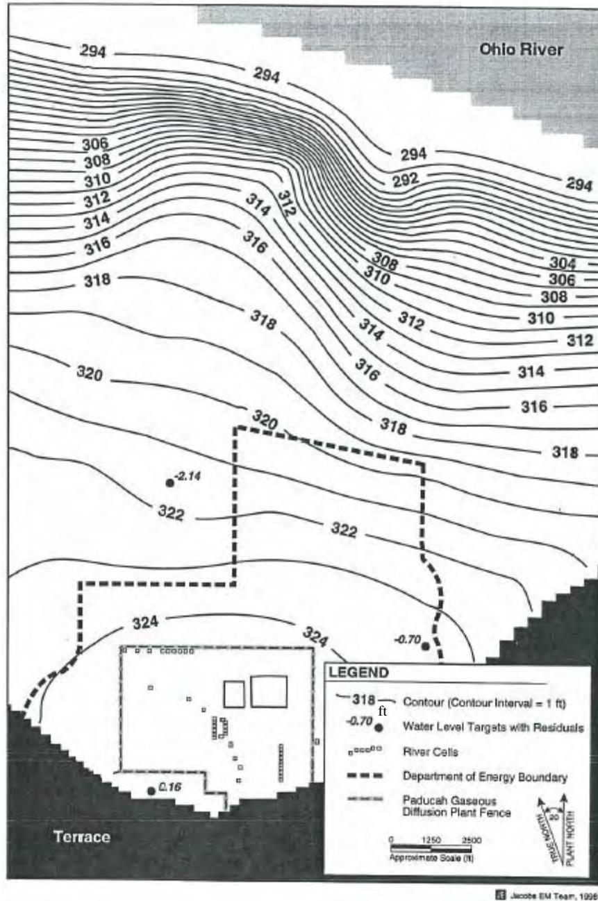
Figure 3.20. Model Layer 4 Predicted Potentiometric Surface
