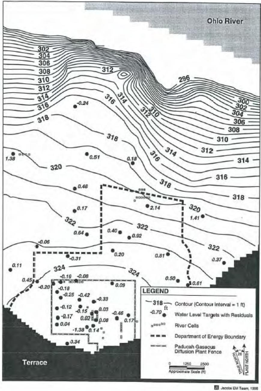
Figure 3.19. Model Layer 3 Predicted Potentiometric Surface
