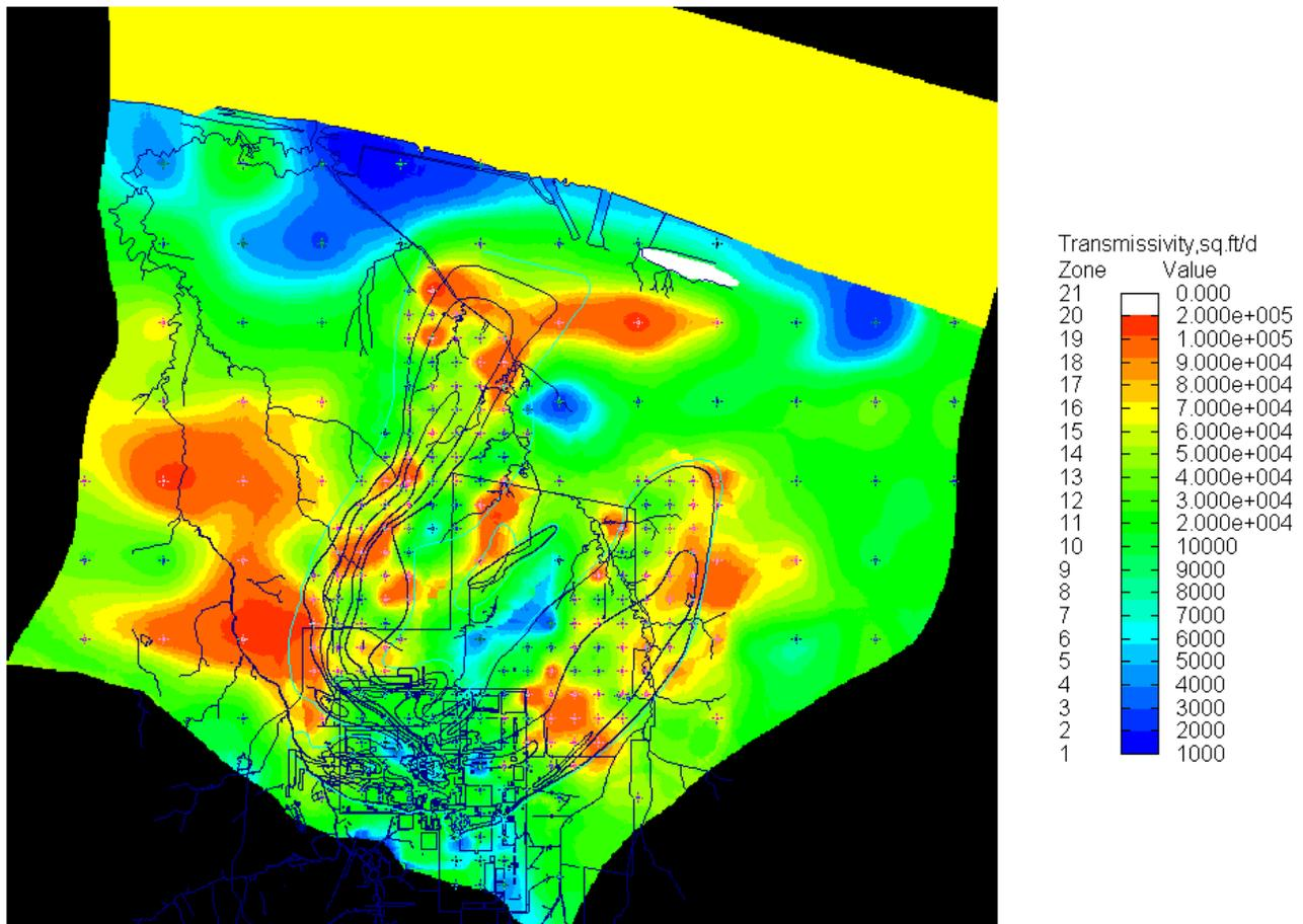
Figure 7.8. PGDP Plant Model-Predicted Transmissivity
