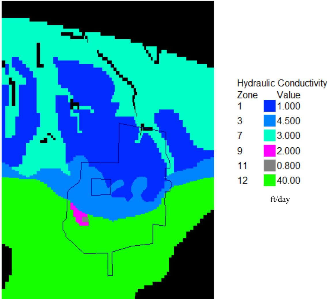
Figure 3.11. Model Layer 1 Hydraulic Conductivity Distribution
