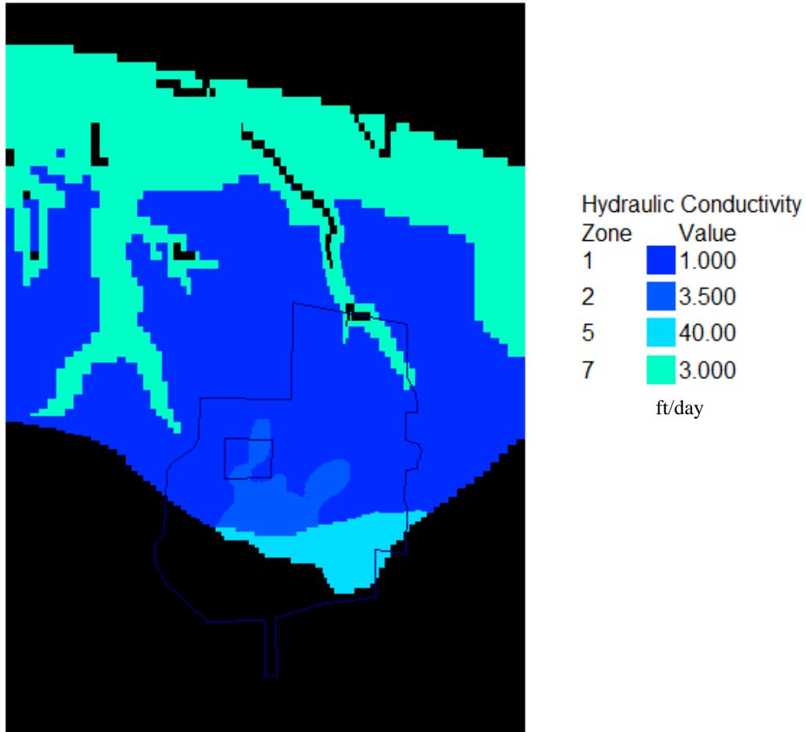
**Figure 3.12. Model Layer 2 Hydraulic Conductivity Distribution**
