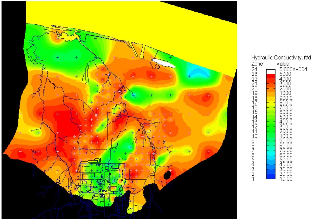
Figure 7.5. Model Layer 1 Predicted Hydraulic Conductivity Distribution
