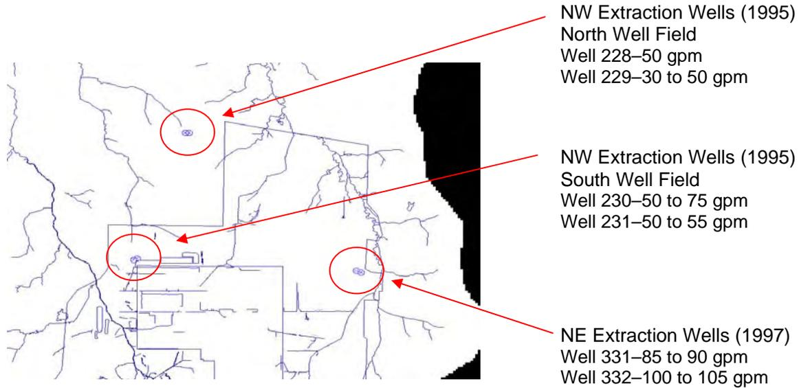
**Figure 4.7. Extraction Well Locations and Pumping Rates**
