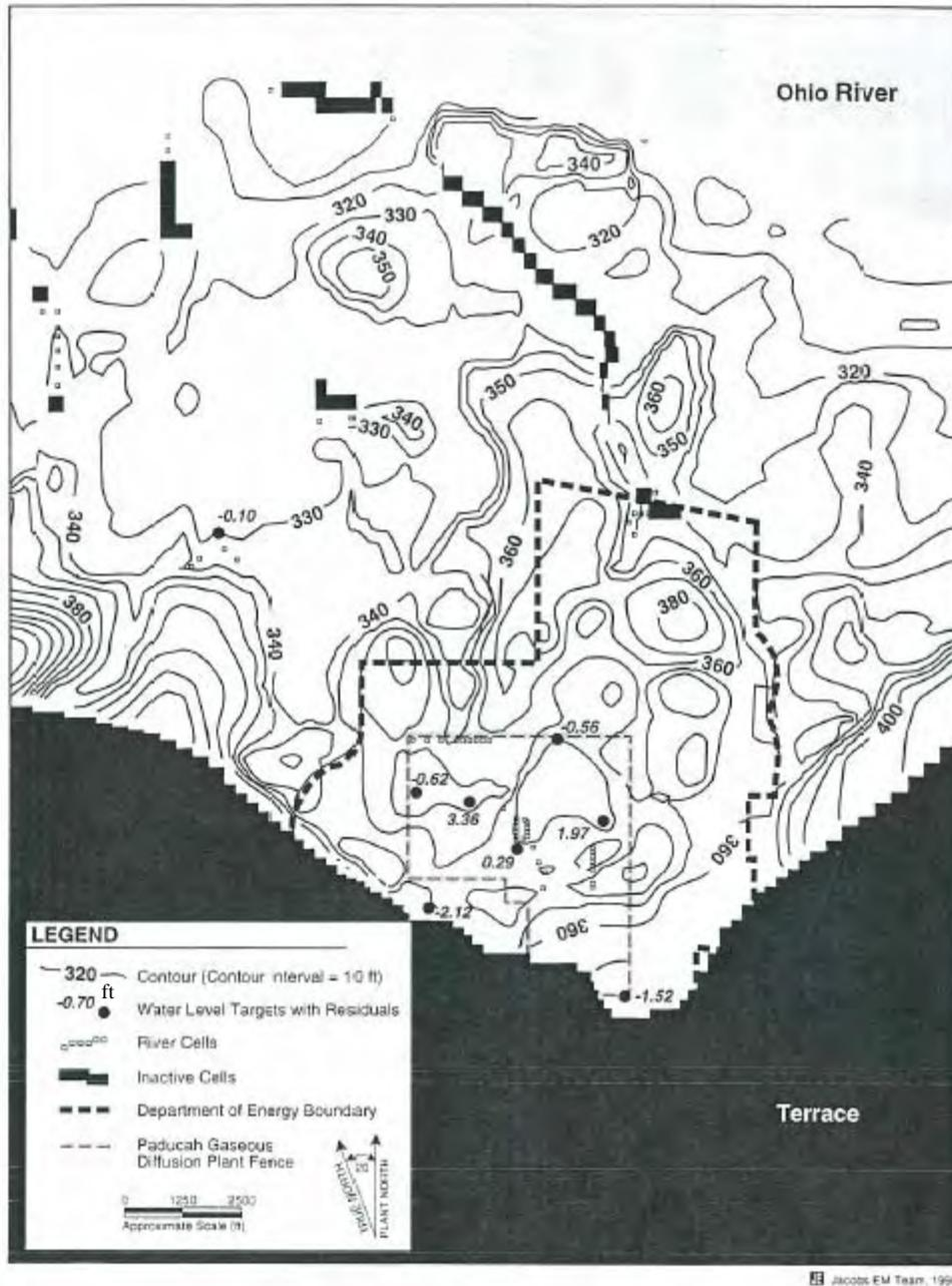
Figure 3.18. Model Layer 2 Predicted Potentiometric Surface
