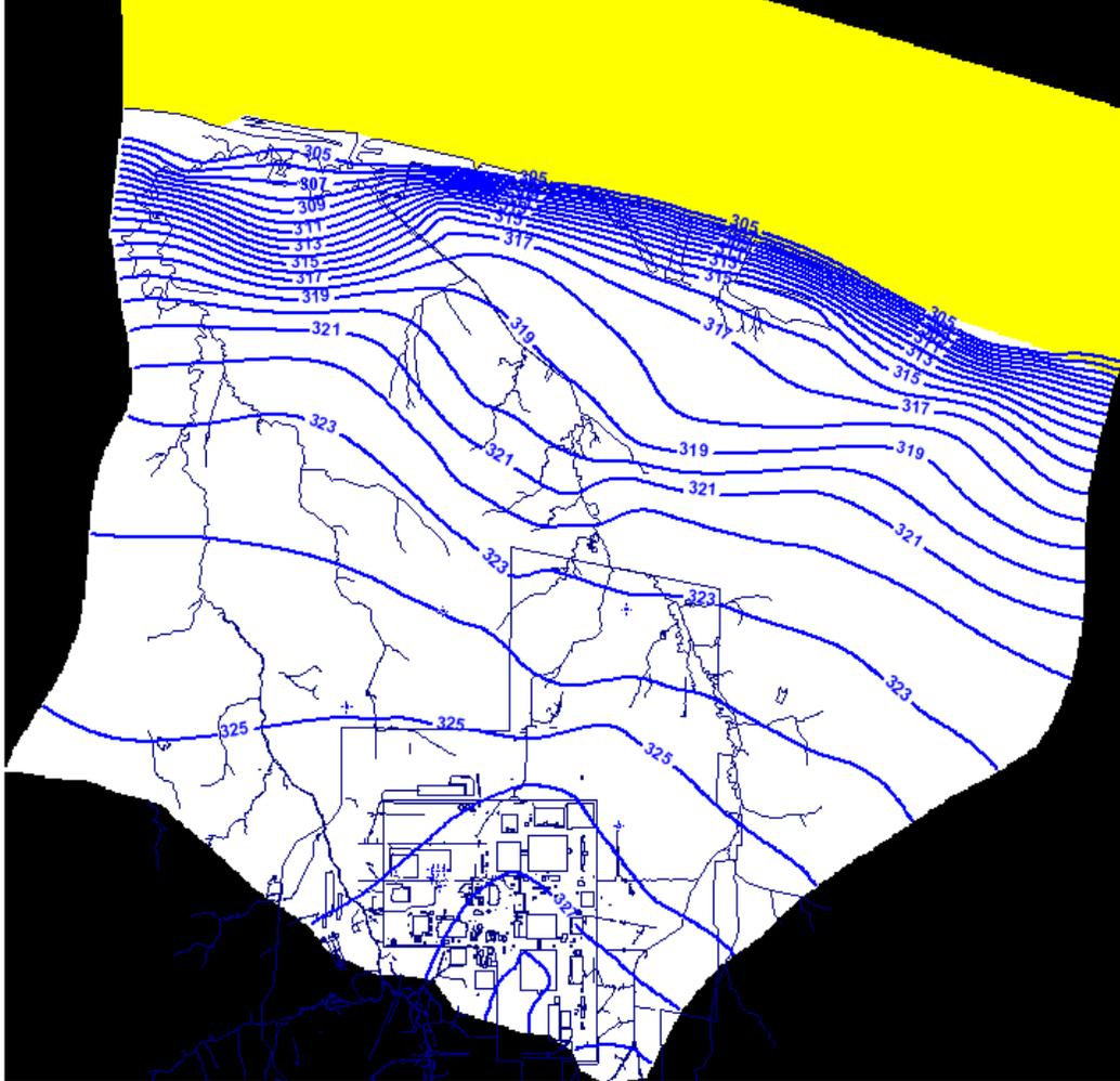
**Figure 7.17. Model Layer 3 Model-Predicted Potentiometric Surface**
