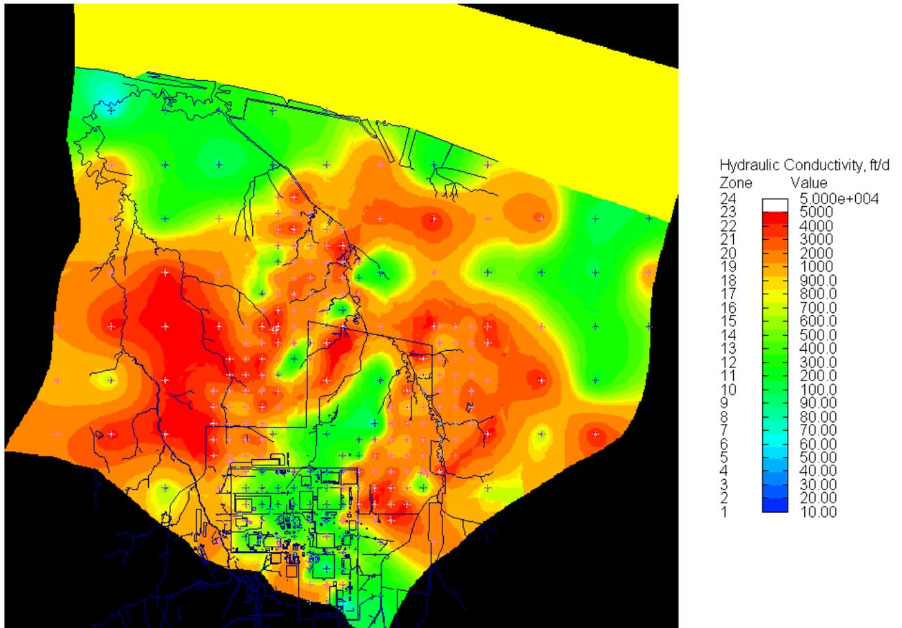
**Figure 7.6. Model Layer 2 Predicted Hydraulic Conductivity Distribution**
