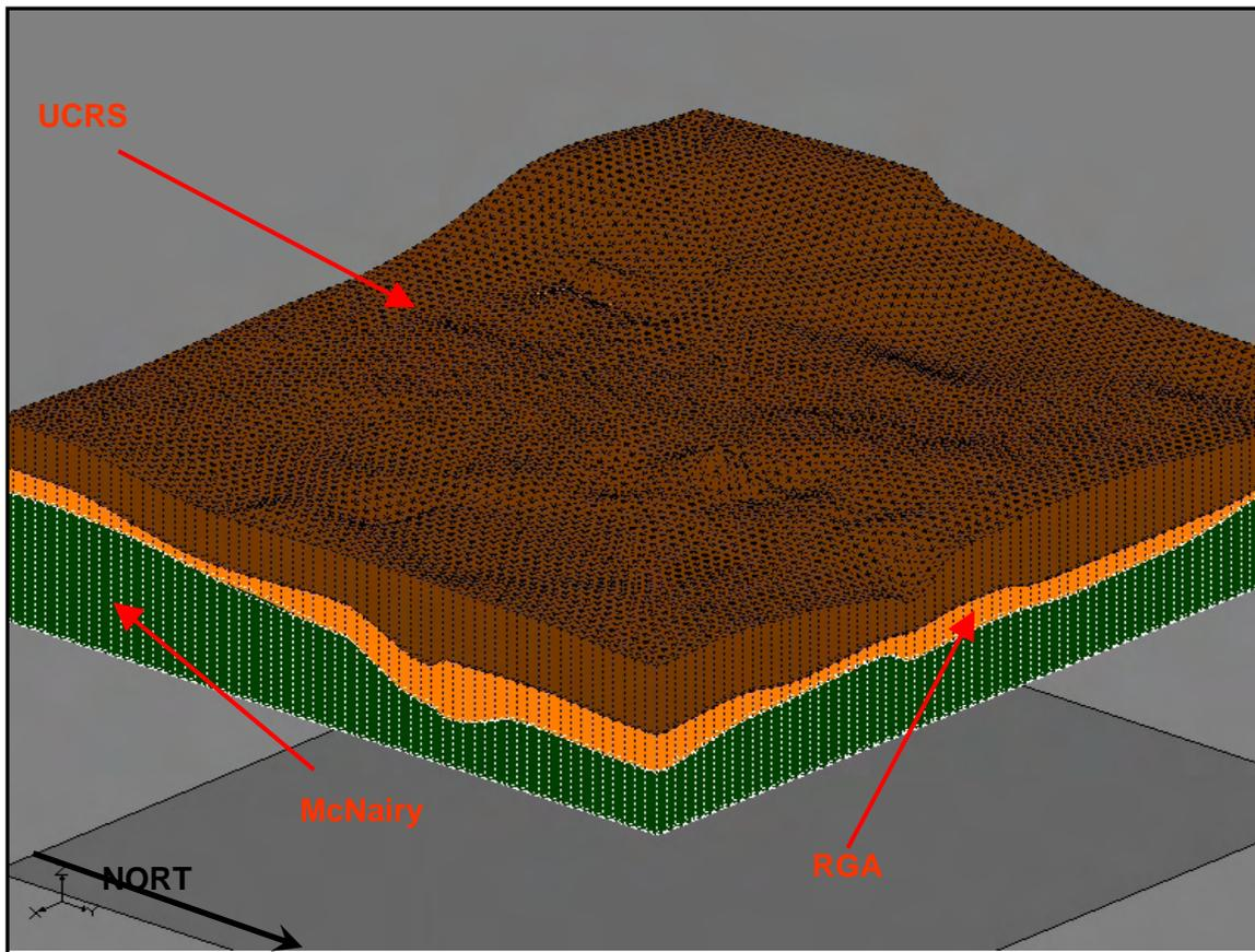
Figure 4.1. PGDP Hydrostratigraphic Units
