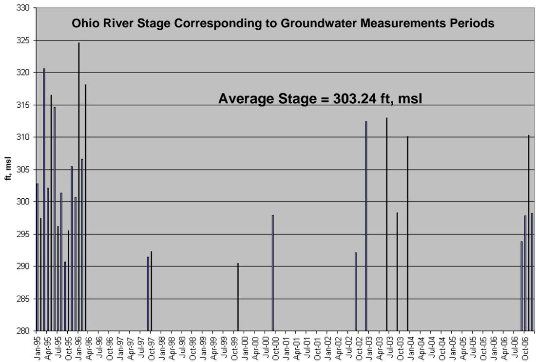
**Figure 4.8. Ohio River Stage Fluctuations**
