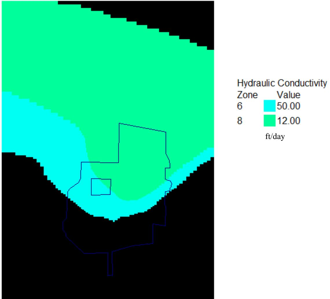
**Figure 3.14. Model Layer 4 Hydraulic Conductivity Distribution**
