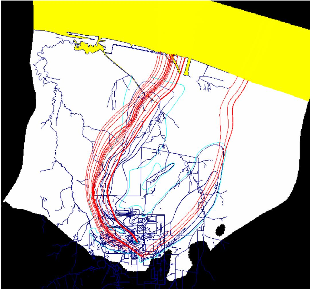
**Figure 7.18. Model-Predicted Plume Flow Paths**
