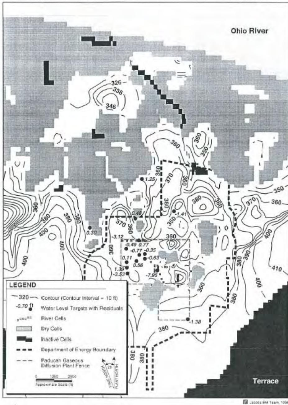
Figure 3.17. Model Layer 1 Predicted Potentiometric Surface
