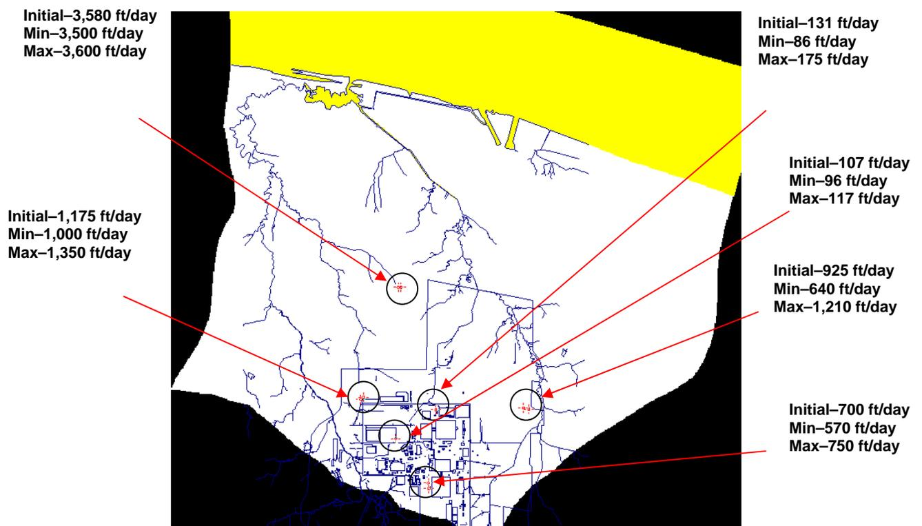
Figure 4.6. RGA Pumping Test Locations and Results
