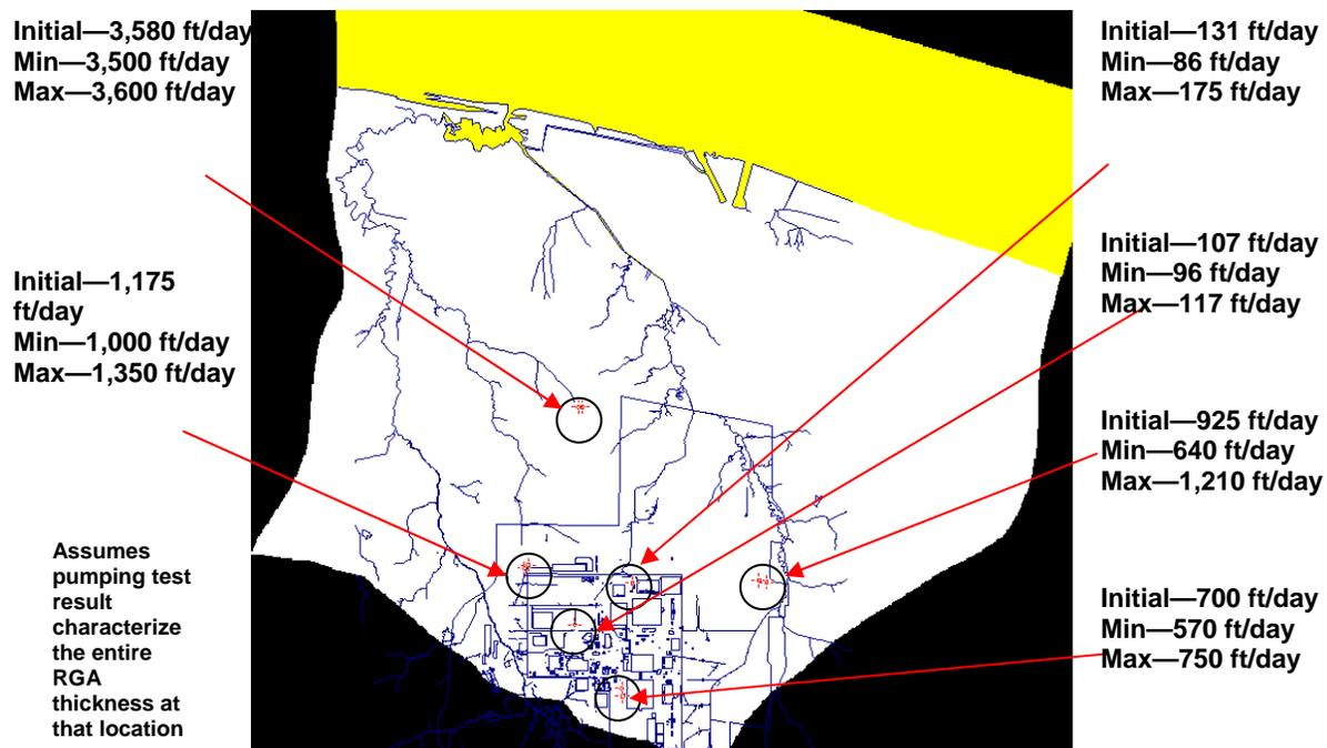
Figure 6.2. Pumping Test Pilot Point Locations
