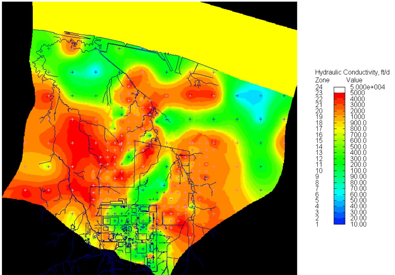
**Figure 7.7. Model Layer 3 Predicted Hydraulic Conductivity Distribution**
