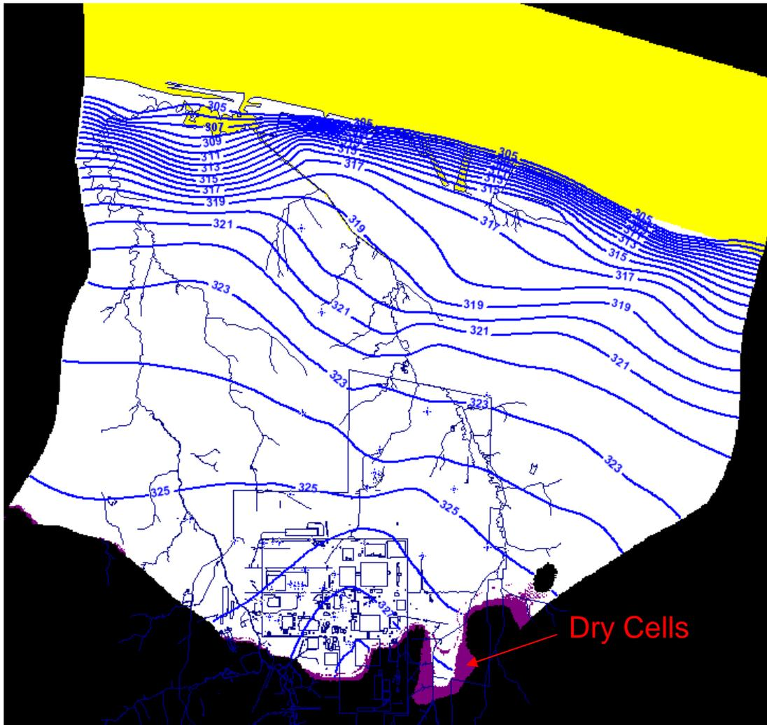
**Figure 7.15. Model Layer 1 Model-Predicted Potentiometric Surface**
