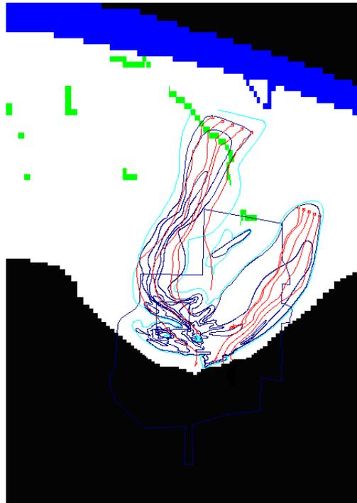
**Figure 3.22. Model-Predicted Plume Flow Paths**
