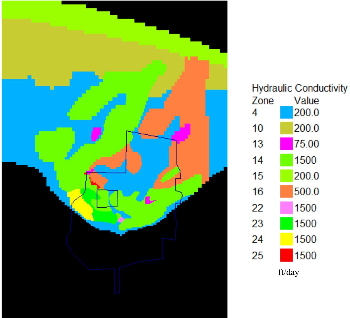
Figure 3.13. Model Layer 3 Hydraulic Conductivity Distribution
