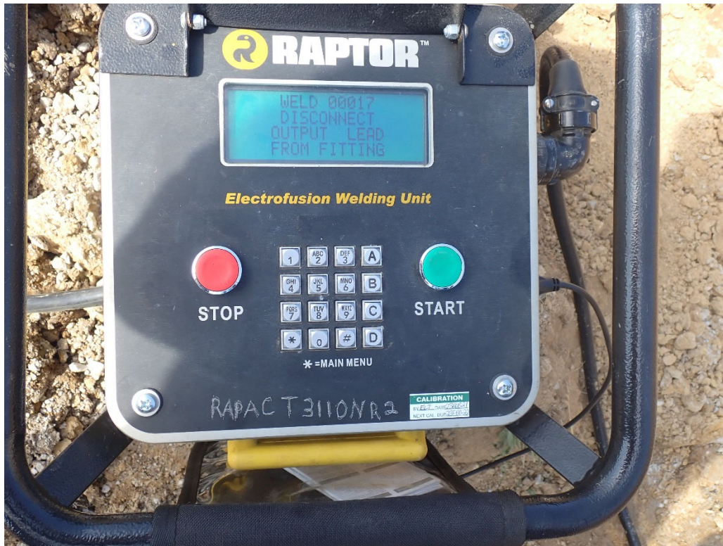
Photo 5, Electrofusion Unit indicating that the weld is completed and the leads can be disconnected
