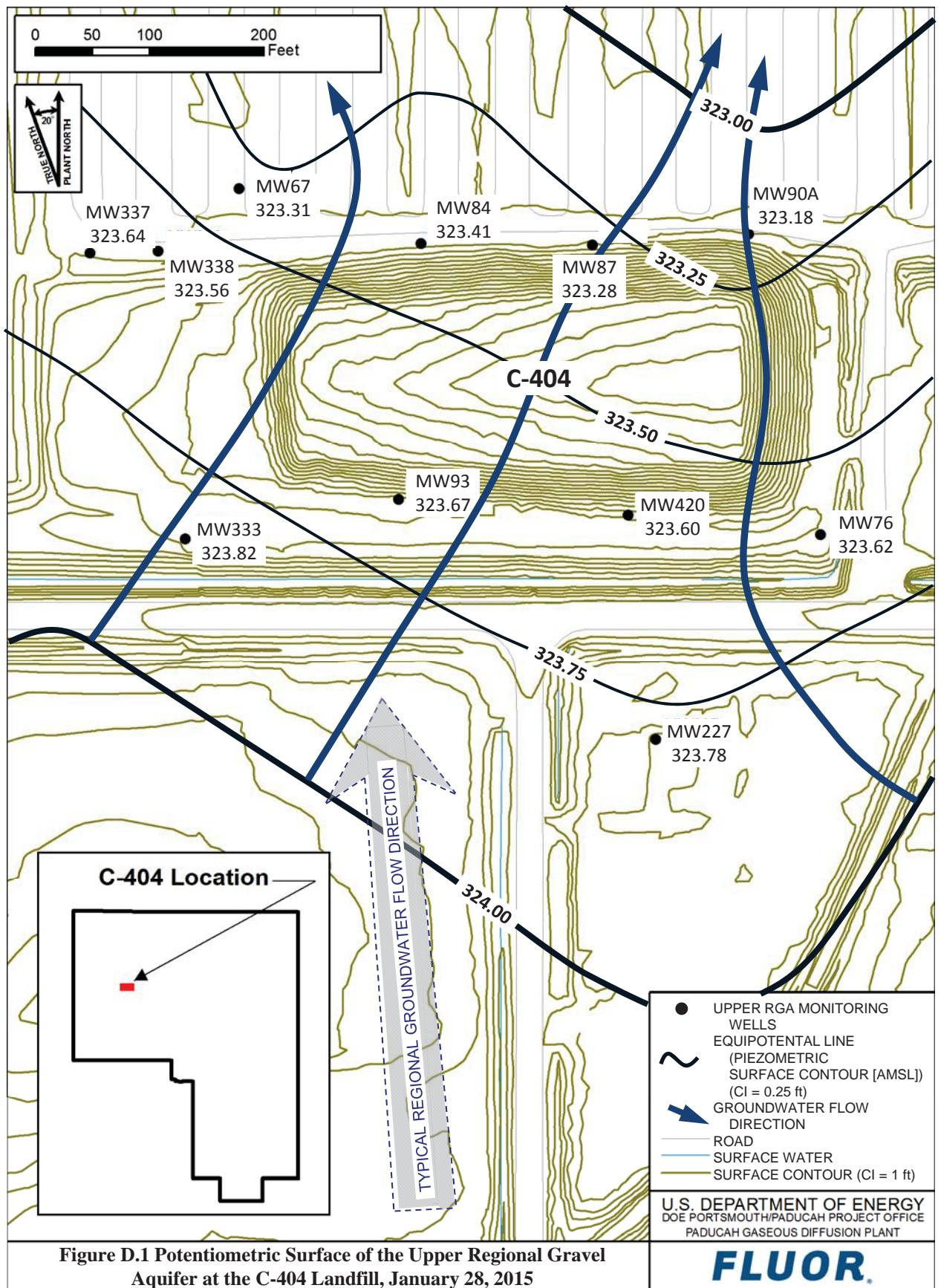
Figure D.1 Potentiometric Surface of the Upper Regional Gravel Aquifer at the C-404 Landfill, January 28, 2015
