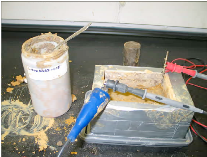
Figure 13: Static testing of soil, C400-RDSI-15 sample
