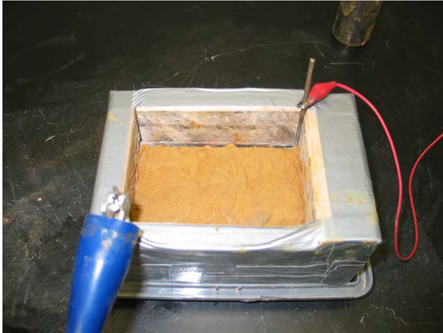
Figure 4: For the C400-RDSI-9 sample, the soil was moist and had a resistivity of 33 \Omega \cdot m
