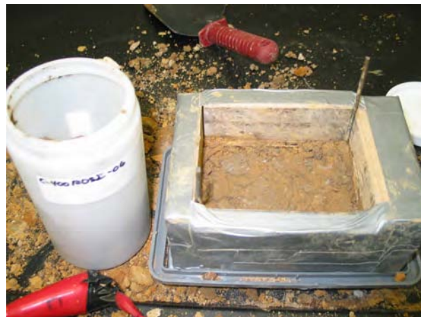
Figure 9: Static testing of soil, C400-RDSI-5 sample
