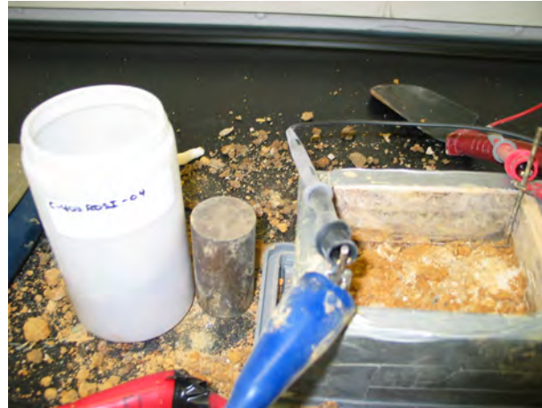
Figure 8: Static testing of soil, C400-RDSI-4 sample
