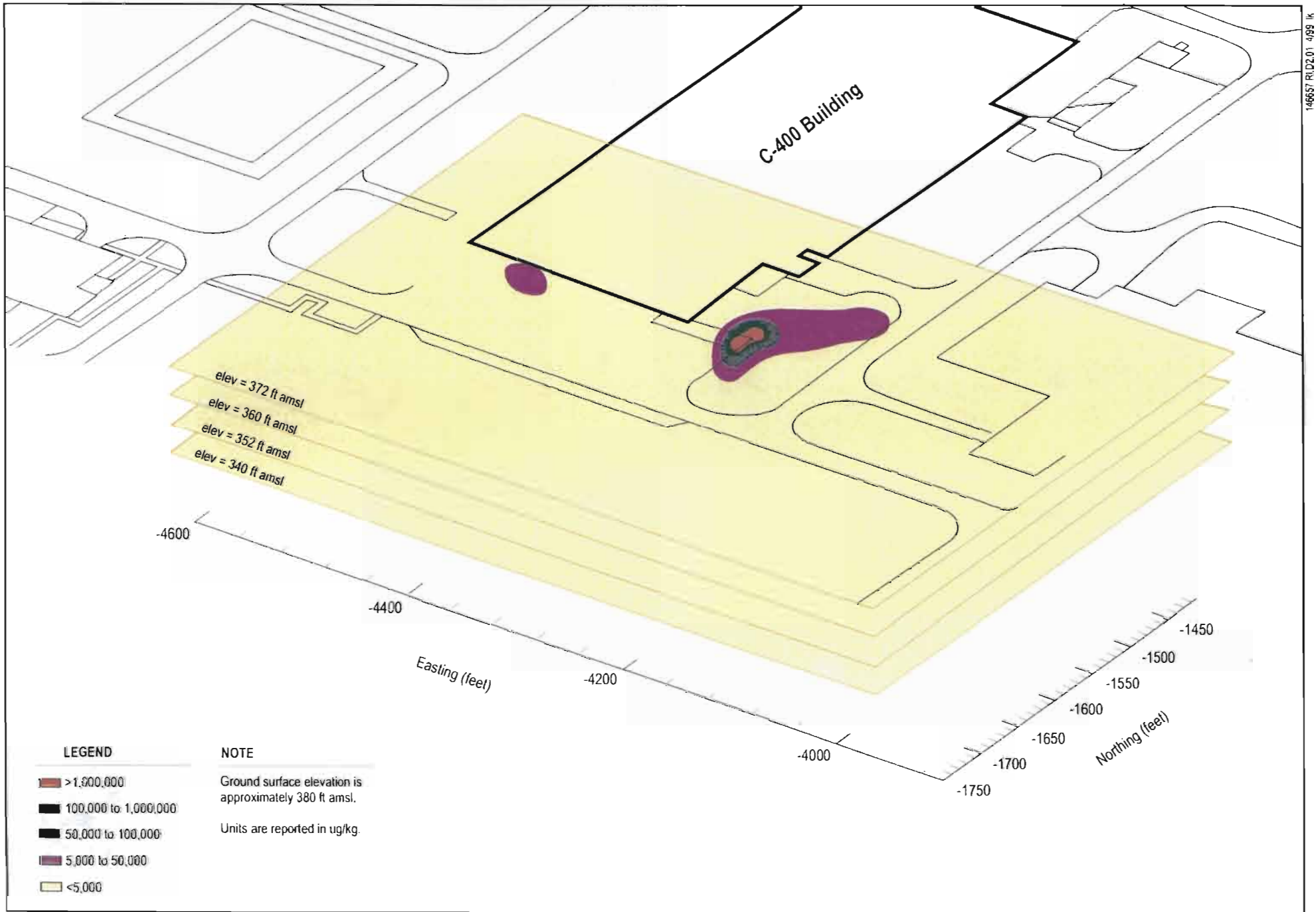
Fig. 4.10.a. Index map of elevation slices through TCE distribution and total concentration of sector 4 and 5 UCRS soil.
