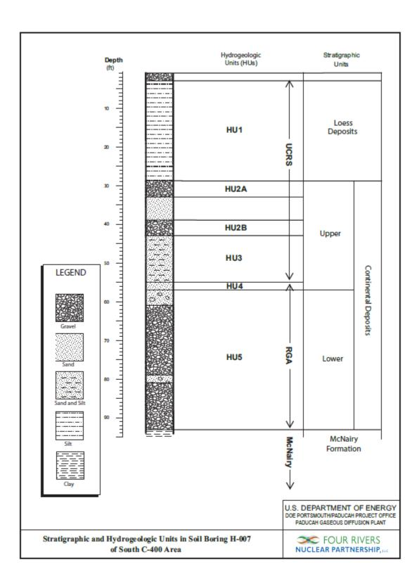
Horizontal flow predominates: hydraulic gradients commonly range between  $10^{-3}$  and  $10^{-4}$  ft/ft northward. Vertical gradients are approximately  $10^{-4}$  ft/ft downward. Hydraulic conductivity of the RGA (ranging from 53 ft/day to 5,700 ft/day) is commonly  $10^4$  X greater than that of the UCRS and commonly  $10^3$  to  $10^5$  X greater than that of the underlying McNairy Formation. The RGA is a semiconfined aquifer.
