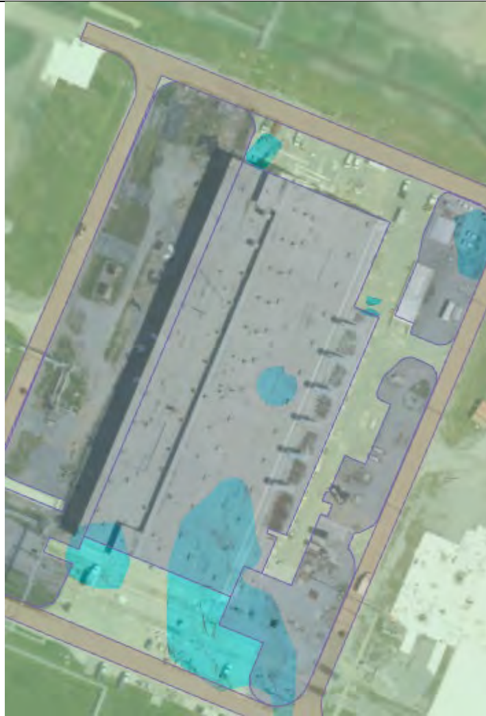
Plan view of EVS model for PID values above 2 \times 10^4
