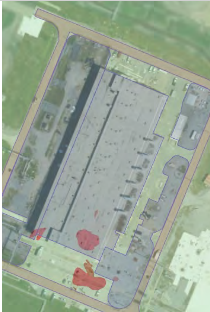
Plan view of EVS model for PID values above 1 \times 10^6
