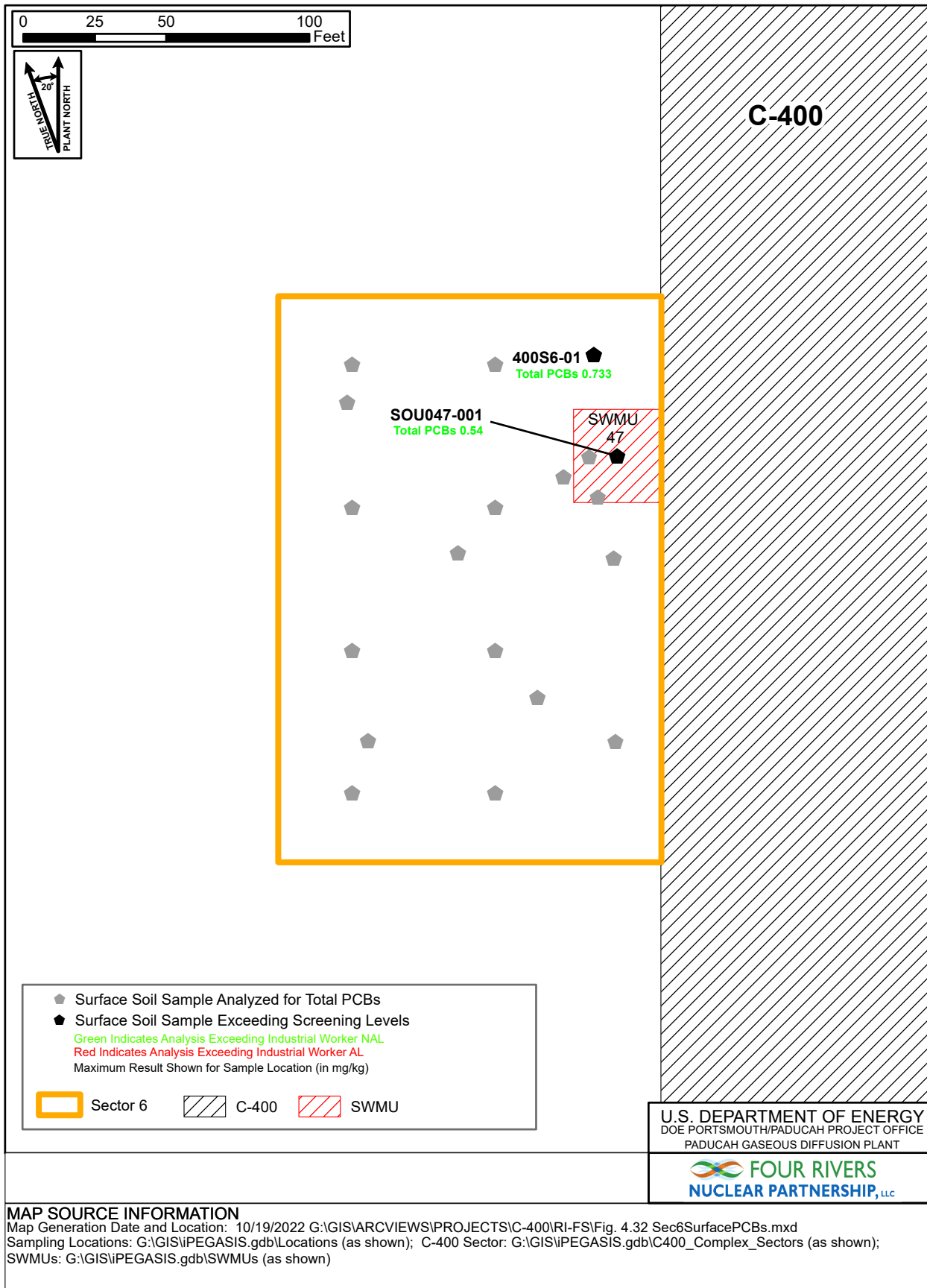
Figure 4.32. Sector 6 Surface Soil Sampling Exceeding Screening Levels for Total PCBs
