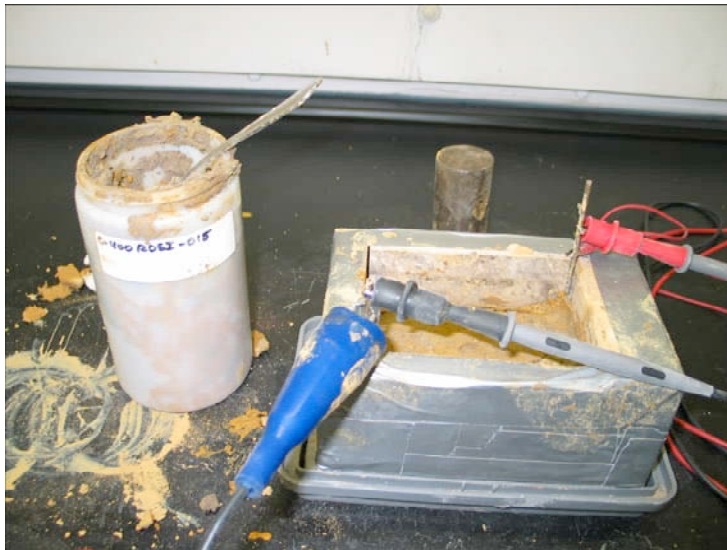
Figure 13: Static testing of soil, C400-RDSI-15 sample
