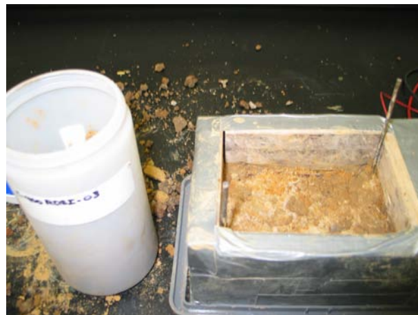
Figure 7: Static testing of soil, C400-RDSI-3 sample
