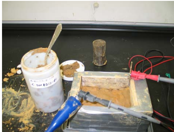
Figure 5: Static testing of soil, C400-RDSI-1 sample
