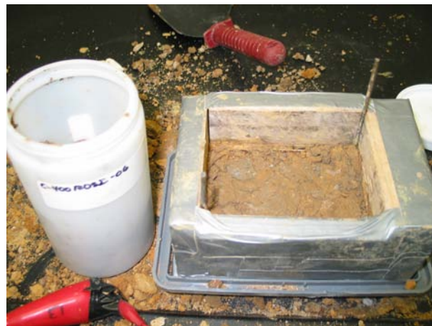
Figure 9: Static testing of soil, C400-RDSI-5 sample
