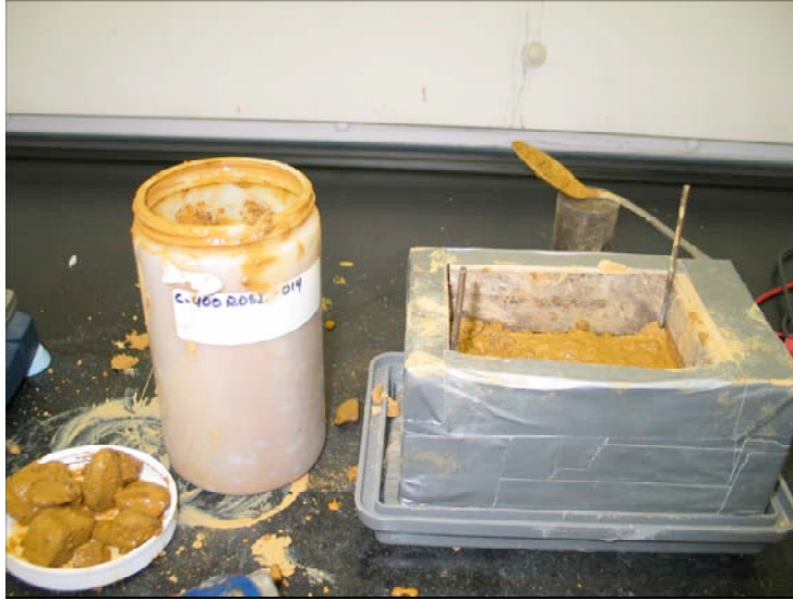
Figure 12: Static testing of soil, C400-RDSI-13 sample
