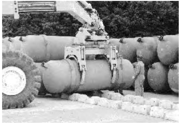
Figure 3.5 Cylinder handler stacking DUF 6 cylinders.
