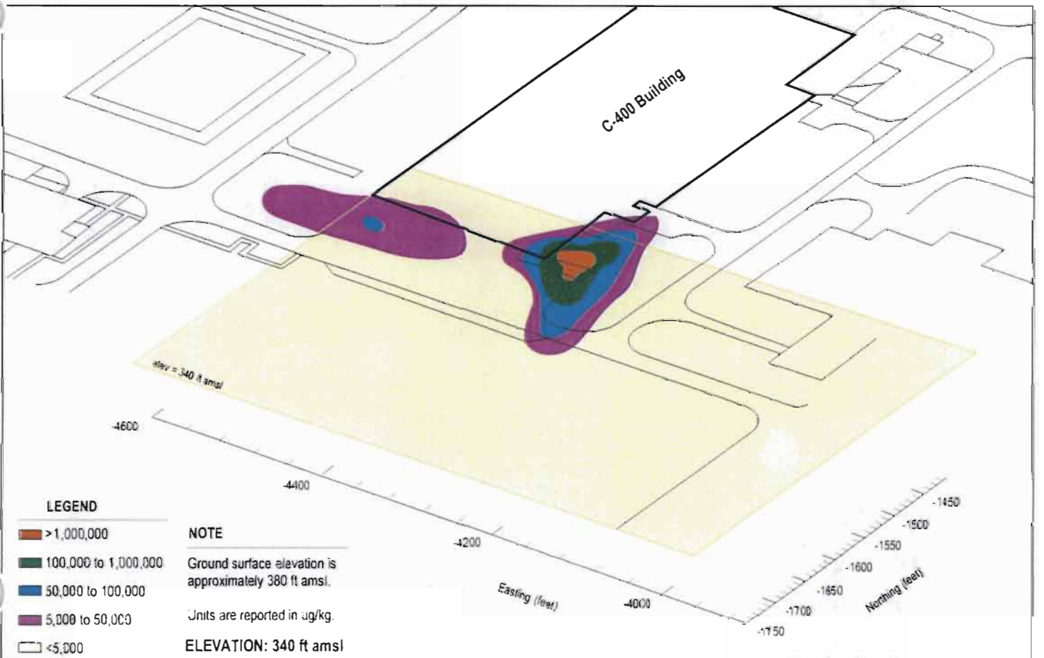
Fig. 4.10.c. 352 ft amsl and 340 ft amsl elevation slice through TCE distribution at sector 4 and 5 UCRS soil.
