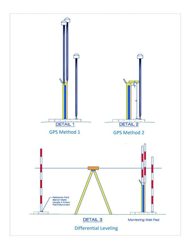
Figure 1. Schematics of Surveying Methods
