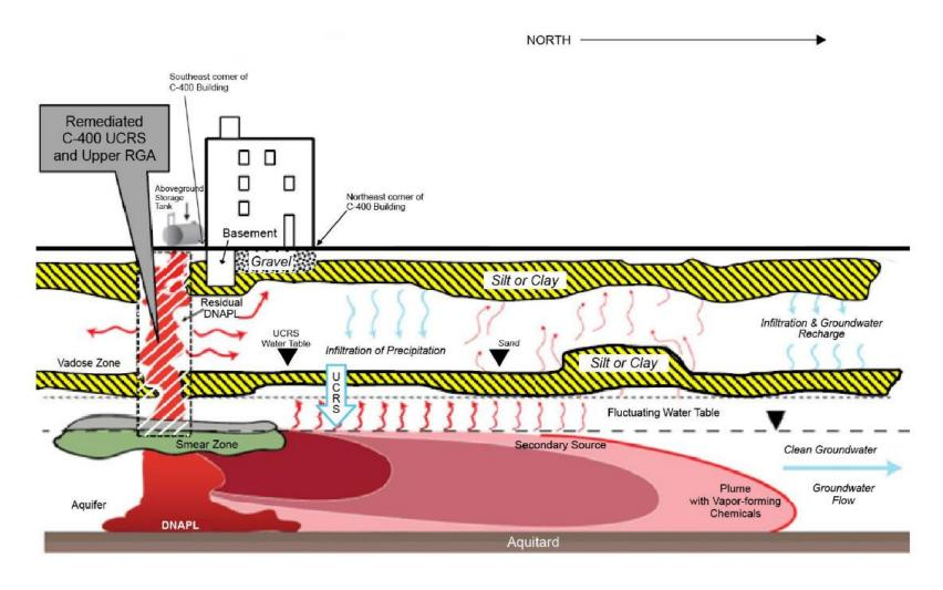
Figure D.2. Hydrogeologic Setting for Conceptual Site Model
