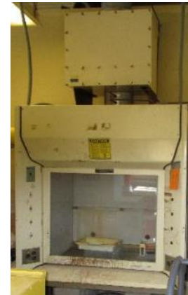
Laboratory Fume Hood
