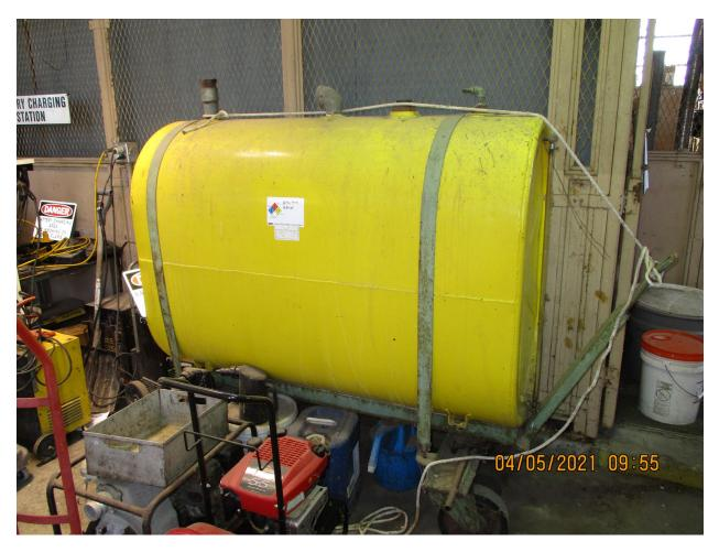
Figure 11. Ethylene Glycol Storage Tank
