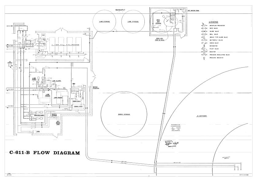
Figure A.5. Engineering Drawing E-P-U-2.0-28M (C-611-B Flow Diagram)
