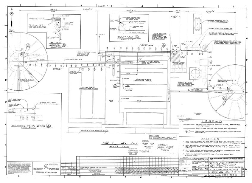
Figure A.6. Engineering Drawing M5E-14782-B (Chemical Feed System Layout Associated with C-611-B and C-611-B1)
