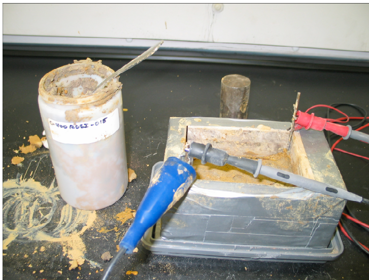
Figure 13: Static testing of soil, C400-RDSI-15 sample
