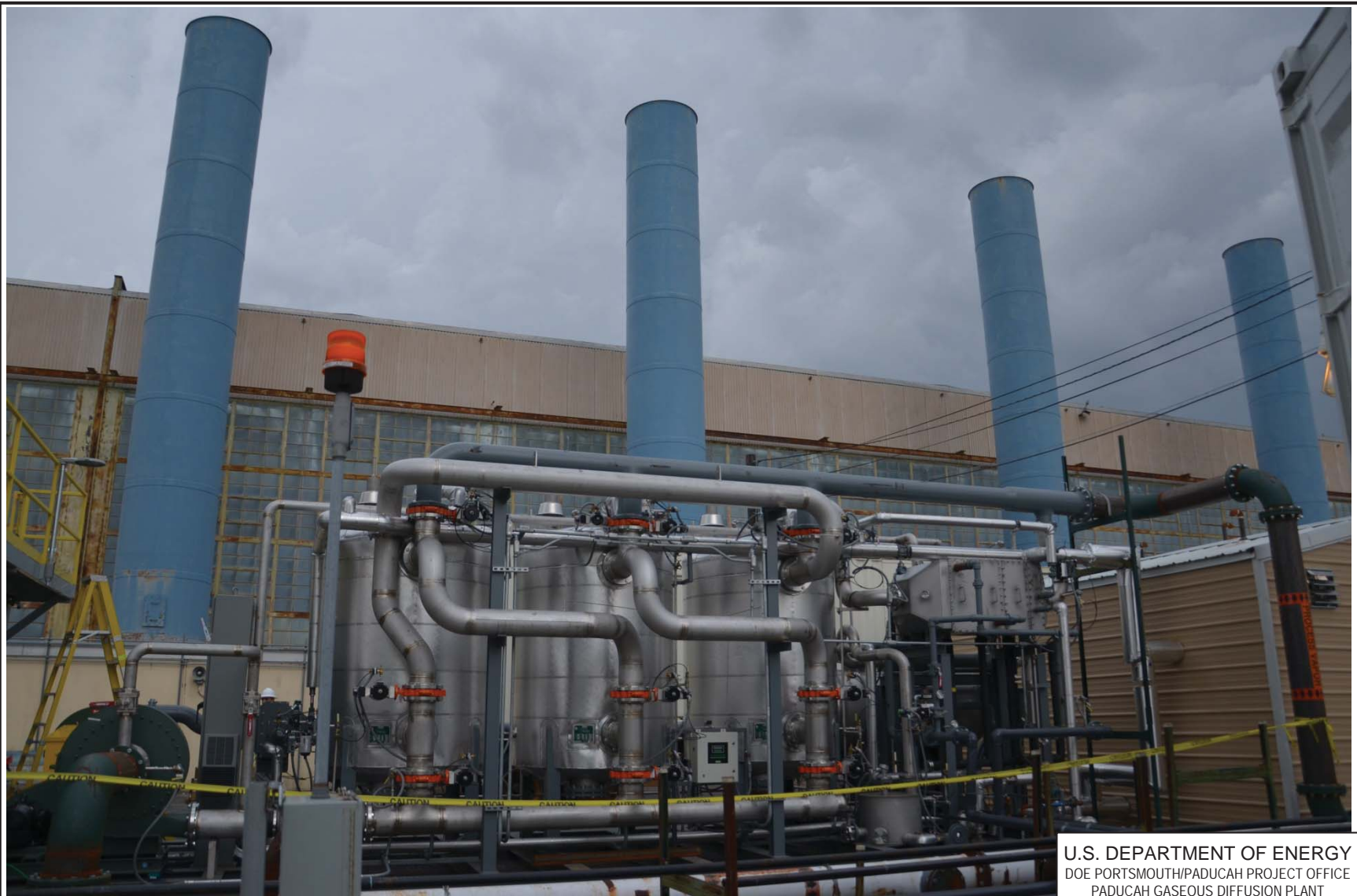
Figure 5.16. C-400 Phase IIa Carbon Regeneration Component
