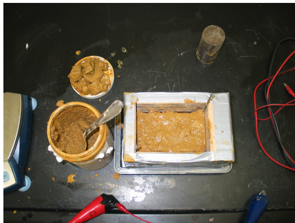
Figure 11: Static testing of soil, C400-RDSI-11 sample
