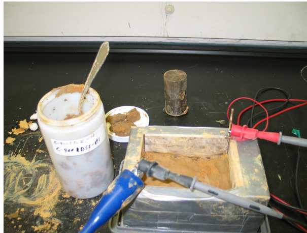
Figure 5: Static testing of soil, C400-RDSI-1 sample
