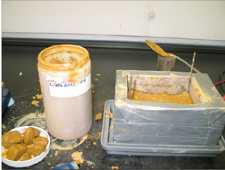
Figure 12: Static testing of soil, C400-RDSI-13 sample
